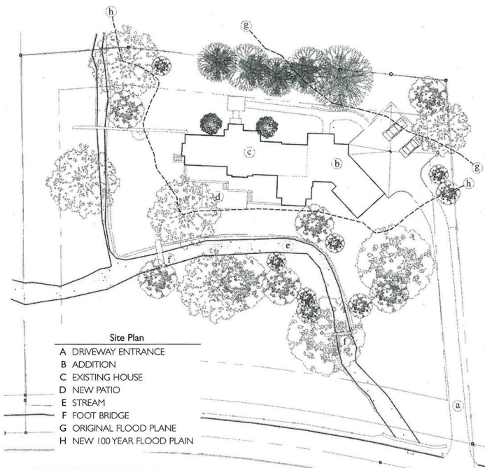
The site plan illustrates how the angled addition responds to the stream and flood plain. New footbridges link the grounds of the main house to the wooded landscape opposite the stream.
